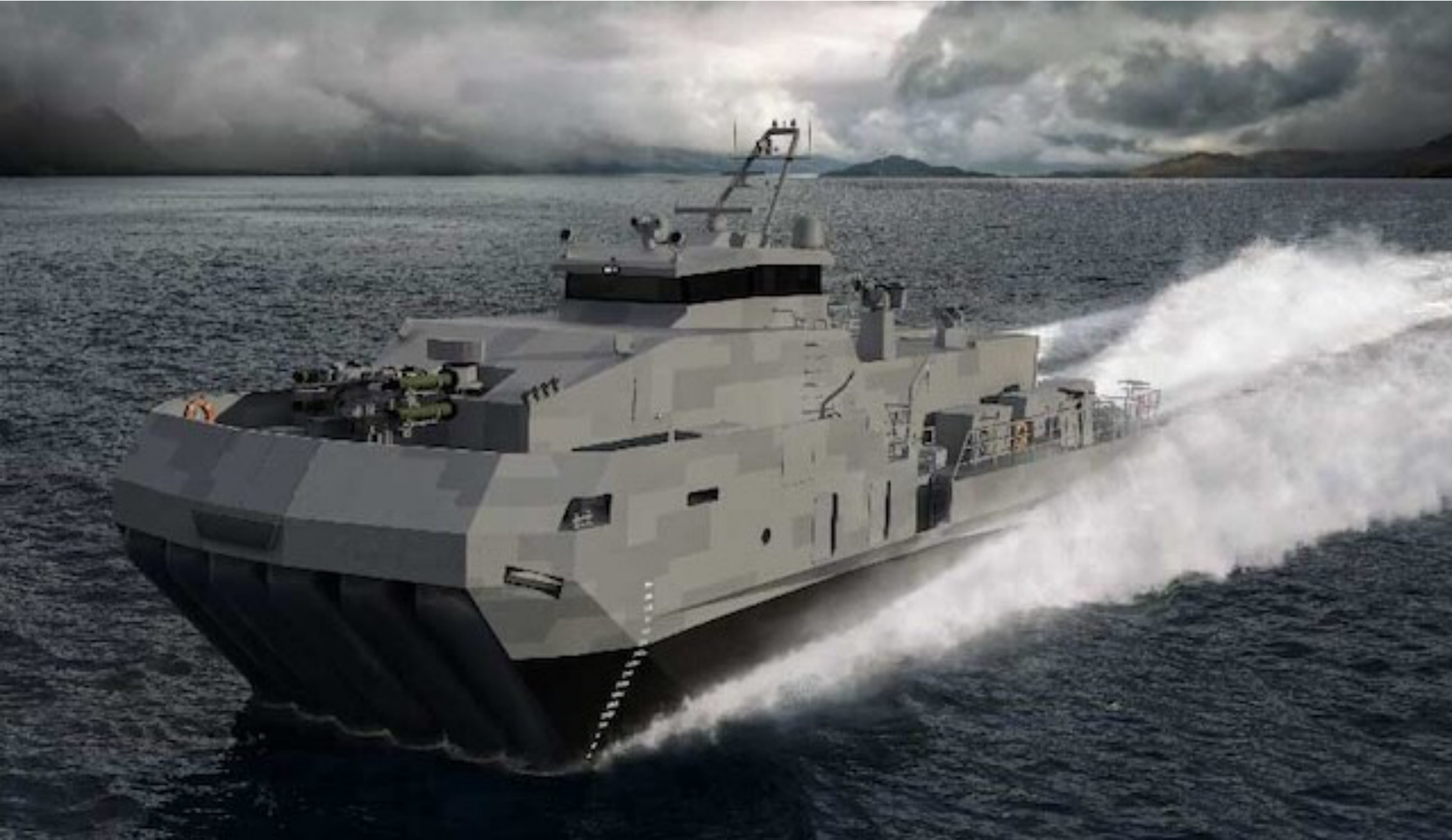
The 36-meter (118') Bengal-MC's versatile air-cushion catamaran design aligns directly with the Navy and Marine Corps' MASC requirements. Bordelon Marine and Eureka Naval Craft rendering
