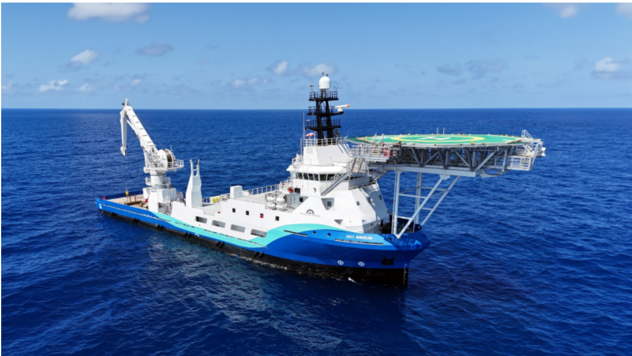
The M/V Lilly Bordelon was rebuilt from a DP-2 PSV hull into an ultra-light intervention vessel for subsea inspection, maintenance, repair, and light construction work. Bordelon Marine photo.
